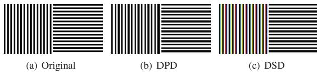
Fig. 3. (a) original image (b) result of Direct Pixel-based Downsampling (DPD) (c) result of Direct Subpixel-based Downsampling (DSD)
