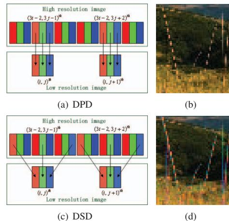
Fig. 2. (a) Direct Pixel-based Downsampling (DPD) (b) result of DPD where “grass” is broken (c) Direct Subpixel-based Downsampling (DSD) (d) result of DSD where “grass” is continuous but with color fringing artifacts
