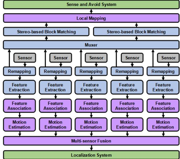
Figure 2: The block diagram of *Guidance*'s built-in functionalities: the blocks with gray, blue, purple and green colors stand for system inputs, FPGA-based hardware kernels, ARM-based software kernels and system outputs respectively.
