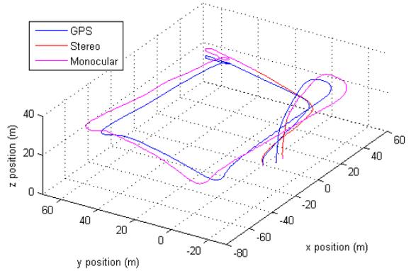
Figure 4: The large-scale performance of Guidance’s built-in visual odometer: the trajectories with blue, red and pink colors stand for the positional observation from GPS, stereo visual odometer and monocular visual odometer respectively. Notice that monocular method is only used at extremely low and extremely high altitude, therefore the pink color is only seen in part of the trajectory.
