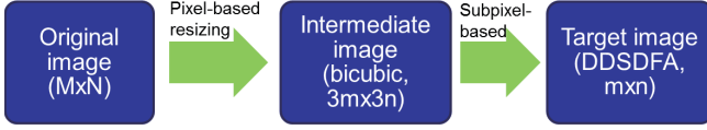
Fig. 2: Conventional arbitrary subpixel downsampling: bic+DDSDFA. First we do bicubic resizing (pixel-based), then we do subpixel downsampling (DDSDFA).
